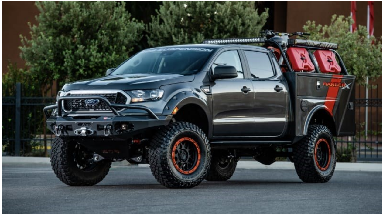
Figure 9: The aftermarket aggressive front end and increased ride height of this vehicle is dangerous to pedestrians and cyclists. The bull bar is angled down which will force a pedestrian underneath the vehicle during a collision. Vision Zero will not be achieved while Australia's vehicle registration standards continue to allow such vehicles to exist on public roads.
