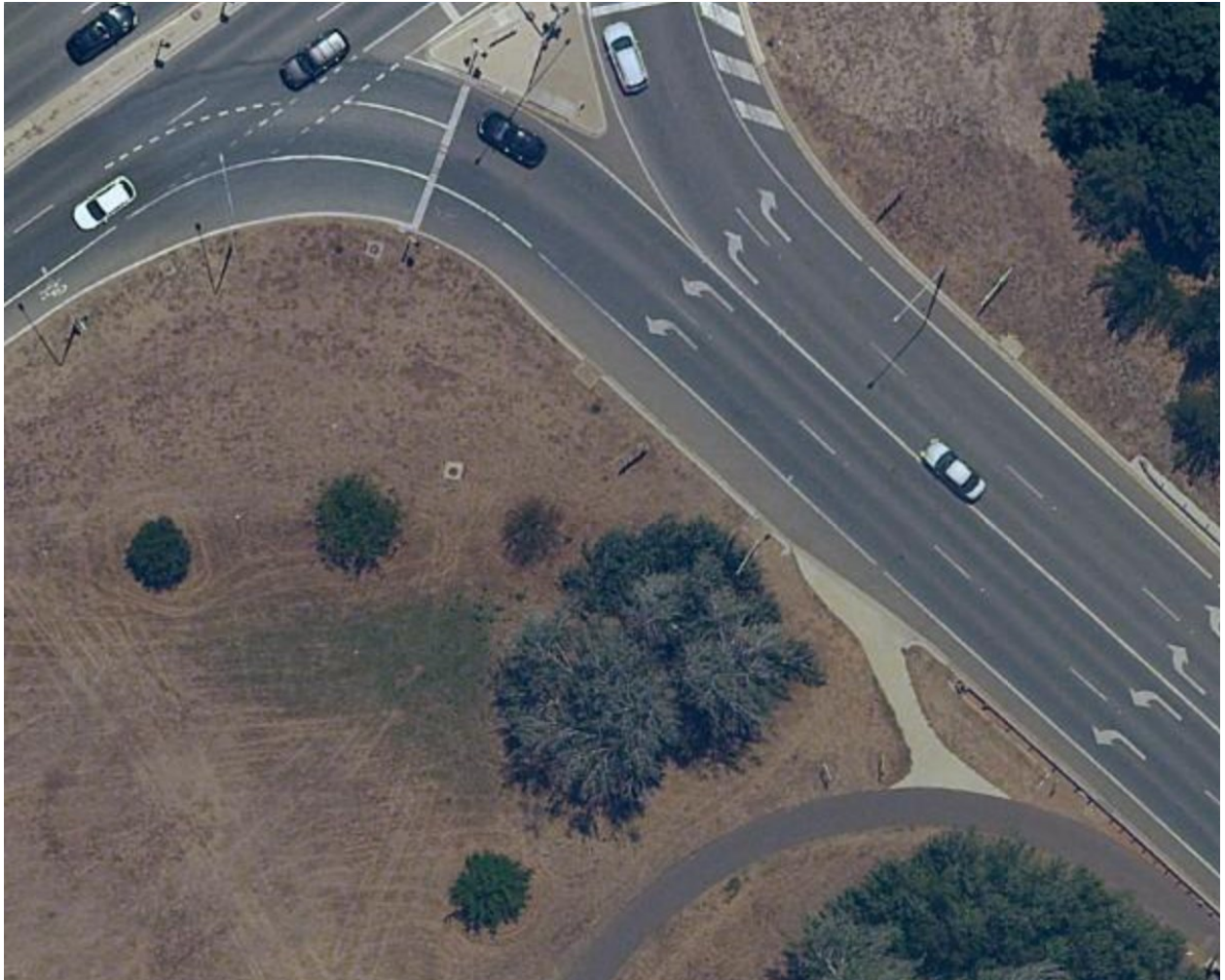
Figure 2: New Australian infrastructure feeding vulnerable road users to a section of road where risk of being run over by a truck trailer is possible. Note the bicycle symbol painted on the road near the stop line has been run over so often, it is now barely visible.
