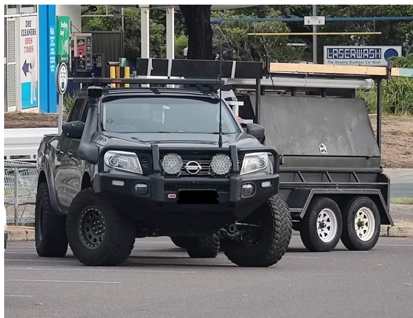
Figure 10: This tradesman's ute above, photographed in an Australian suburban carpark, has many modifications including aggressive bumper bar, increased ground clearance, large wheels which protrude past frame of the vehicle. All of these modifications increase risk to vulnerable road users and have no place being permitted on urban roads if Australia is to achieve Vision Zero.
