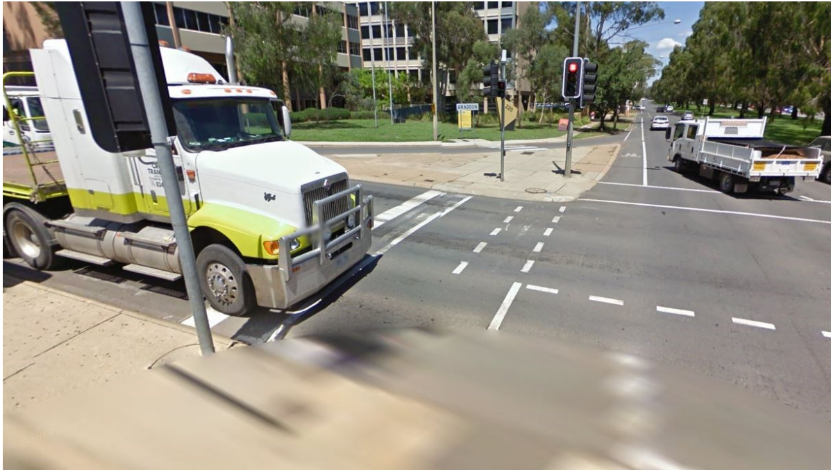
Figure 7: Google Street view image of an Australian intersection. Even if the driver of this truck had correctly stopped before the stop line, it is unlikely they would have been able to keep the entire pedestrian area in front of them in full view.
